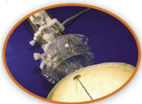
Fig. 7. Frameless stereotaxic surgery enabled by the Nexframe system. Developed to eliminate the need for heavy stereotaxic frames, as illustrated in Fig. 1, which are secured to the patients skull with sharp pins. (Image courtesy of Medtronic Neuromodulation Division.)
