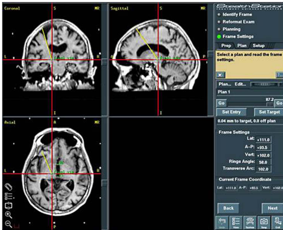
Fig. 4. Medtronic's StealthStation software application provides a graphical user interface for the physician to determine stereotaxic coordinates of target (intersection of red lines) and the best track for electrode penetration (yellow line). (Image courtesy of Medtronic Neuromodulation Division.)
