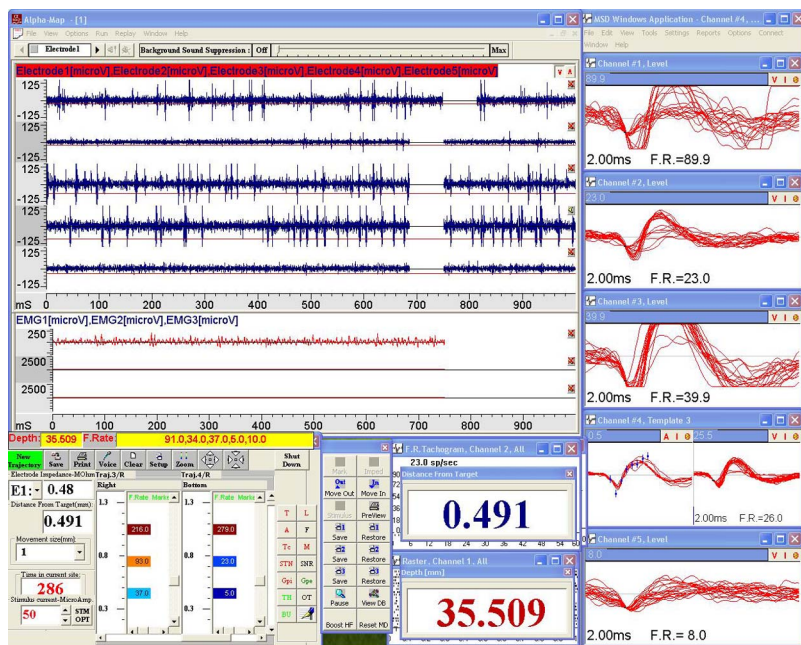
Fig. 6. Alpha-Omega’s Alpha-Map allows monitoring intraoperative microelectrode recordings. Shown here are simultaneous microelectrode recordings from the thalamus, EMG recordings, and extracted neural spikes from selected channels.
